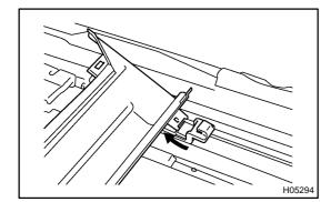
(b) Remove the rear drip channel as shown in the illustration.
