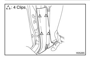
(b) Using a screwdriver, remove the center pillar lower garnish as shown in the illustration.
