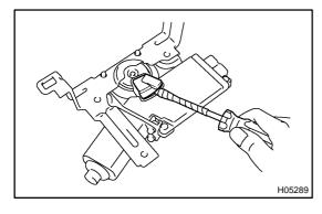
(c) Using a screwdriver, remove the cam plate cover. HINT:
