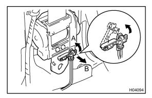
(a) Disconnect the pretensioner connector in the order "A" and "B" as shown in the illustration.
