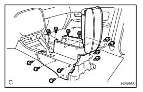
(b) w/ Disc player changer: Install the rear console box with the 4 bolts and the 8 screws.
