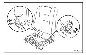
(d) Remove the 4 bolts and the seatback assembly.
