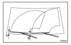
(c) Adjust the installation position of the wiper arms to the positions shown in the illustration.
