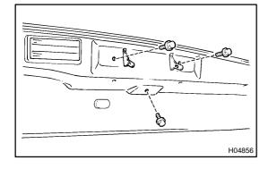
(b) Remove the 3 bolts and back door outside handle assembly.
