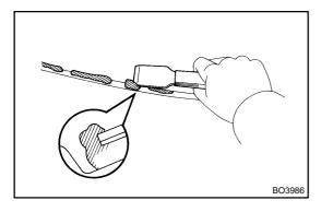
(c) Use a scraper to remove any excess or protruding adhesive.
