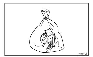
(e) Dispose of the front seat outer belt (with seat belt pretensioner).
