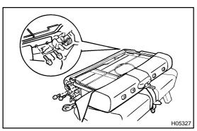
(d) Remove the 4 bolts and seatback assembly.
