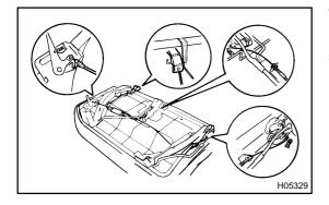
7. REMOVE NO. 1 FOLD SEAT LOCK CONTROL CABLE Remove the 2 clamps and No. 1 fold seat lock control cable as shown in the illustration.
