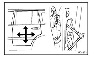
(f) Loosen the body side hinge nuts to adjust.
