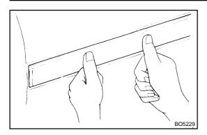
(c) Press firmly on the moulding. Refer to the illustration for the moulding application procedures.
