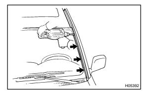
(c) Gently and vertically put the drill to the rivet and cut the rivet flanges.
