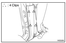
(b) Using a screwdriver, remove the center pillar lower garnish as shown in the illustration.
