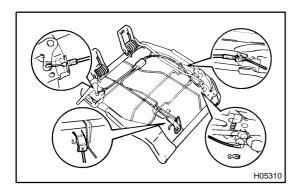
**20. REMOVE NO. 2 FOLD SEAT LOCK CONTROL CABLE** Loosen the clamp and No. 2 fold seat lock control cable as shown in the illustration.
