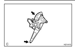
★ At the time of reassembly, apply MP grease to the window regulator.
