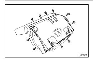
(b) Remove 10 screws and seat cushion under cover sub-assembly.
