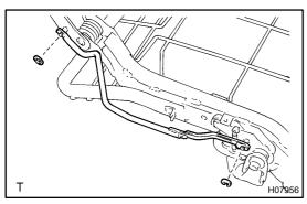
Using a screwdriver, remove the spring nut, E-ring and LH No. 1 seat leg stay.
