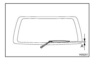
(d) Adjust the installation position of the wiper arm to the position as shown in the illustration.
