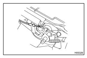
(c) Remove the reclining connecting wire of RH side edge.
