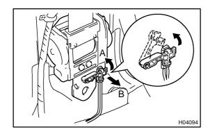
(6) Disconnect the pretensioner connector in the order "A" and "B" as shown in the illustration.
