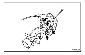
★ Remove the protector, and apply MP grease to the sliding and rotating parts of the door lock.
